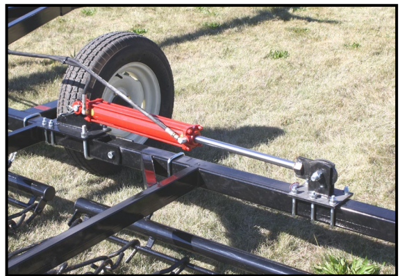
Typical Wing Bracket installation
